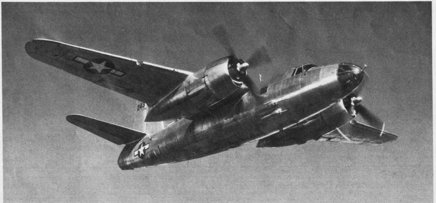
B-26 can still be recognized by shoulder wing, thick body and tall fin and rudder. Rounded tail cone and gun position are now standard.
